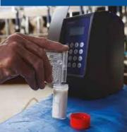
For herds who don't milk record but want to know the cell counts of individual cows (e.g. when investigating a bulk tank cell count problem or checking on individual cow cell counts before drying off) we have a DeLaval cell counting machine at the surgery which can provide same day accurate results.
